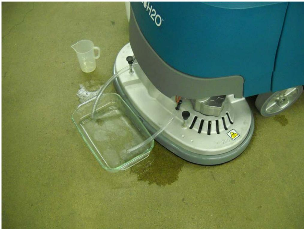
Photograph 4-2: Typical water flow measurement setup
