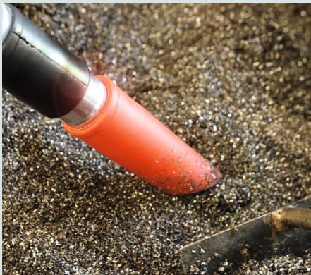
Recovery of metal chips
